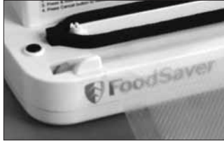
Place Bag on Sealing Strip
