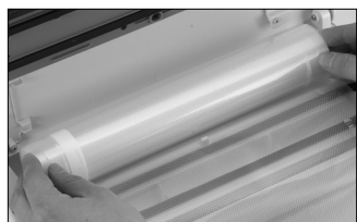
Place Bag in Vacuum Channel
